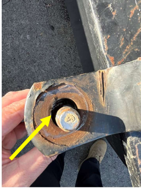
Gap between ball shank and hitch opening.
