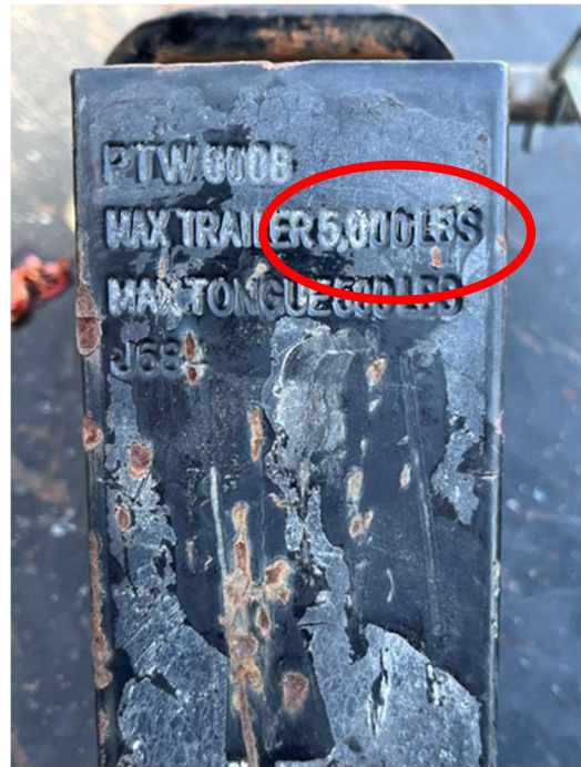
Maximum loads of ball and hitch, 3,500 and 5,000 lbs.
